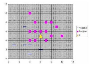
Assume that each case in the training set has two predictor variables, x and y. The cases are plotted using their x,y coordinates as shown in the figure. Also assume that the target variable has two categories, *positive* which is denoted by a square and *negative* which is denoted by a dash. Now, suppose we are trying to predict the value of a new case represented by the triangle with predictor values x=6, y=5.1. Should we predict the target as positive or negative?
